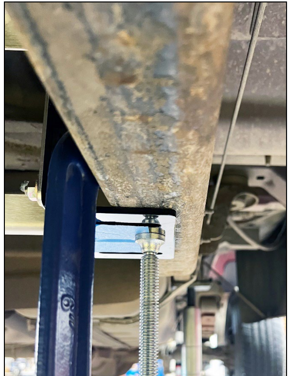
INSIDE / BRACKET EXTENDED AWAY FROM FRAME
